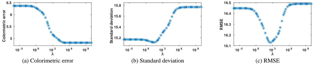
**Fig. 1.** Results of the MSE calculation by Eq. (10) for our proposed TCC matrices with different parameter values. Each result shows the average of all 96 training patches with  $\sigma = 4$ . (a) Colorimetric error, (b) standard deviation of noise, and (c) RMSE. Note that LCC and PCC are equivalent to the cases of  $\lim \lambda \rightarrow 0$  and  $\lim \lambda \rightarrow \infty$ , respectively.
