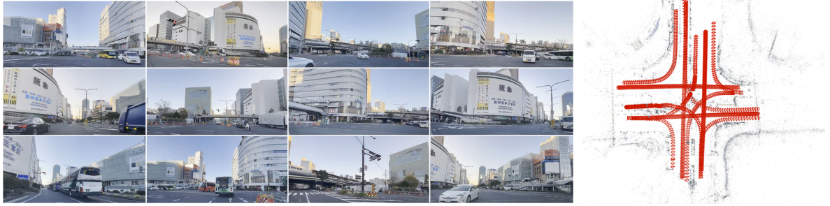
Figure 3: (Left) Sample images of our dataset for an intersection. Each image is from each of 12 video clips. (Right) Estimated camera poses by using COLMAP.
