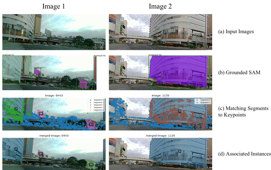
Fig. 3: Visualization of multiple perspectives of the 3D object with the key stages in the proposed processing pipeline. (a) Input source image. (b) Grounded SAM output. (c) COLMAP 2D keypoints overlaid on the masks and linked to their corresponding 3D point IDs via track associations. (d) associated mask sets forming complete building instances by grouping segments that share common 3D points and merging building instances (building 3 in (c) merged into building 2 in (d)).
