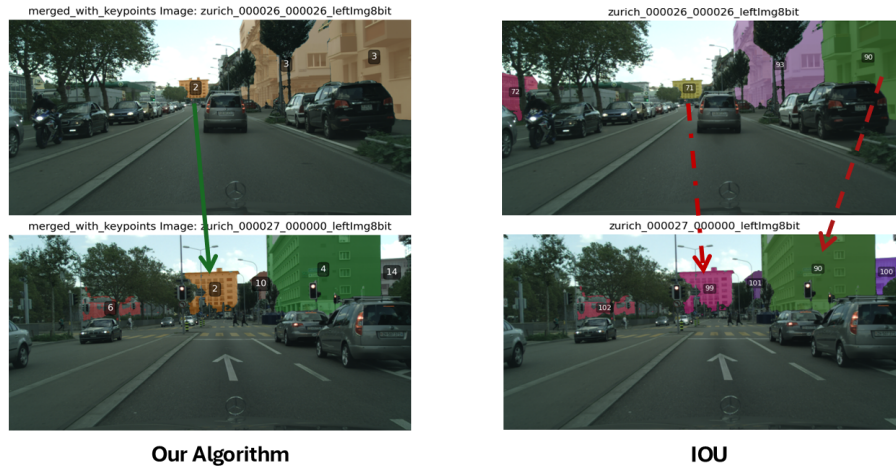
Fig. 6: Typical errors generated with motion tracking compared to our method. The two frames (top and bottom) are from separate sequences in Dataset 2 . Our method correctly assigns ID 2 to the building in the center of the frame (marked with a green arrow). IoU is wrong both in the ID assignment for this building (dashed-dotted red arrow) and incorrectly assigns the same ID to two separate buildings at the edge of the frame, inducing ID spillover (dashed red arrow).
